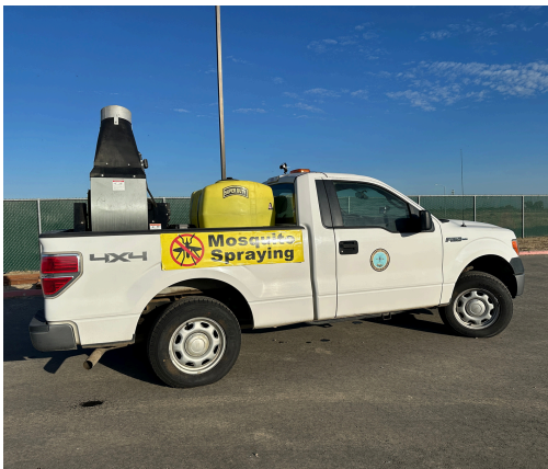
A-1 mist sprayer used for WALS applications.
