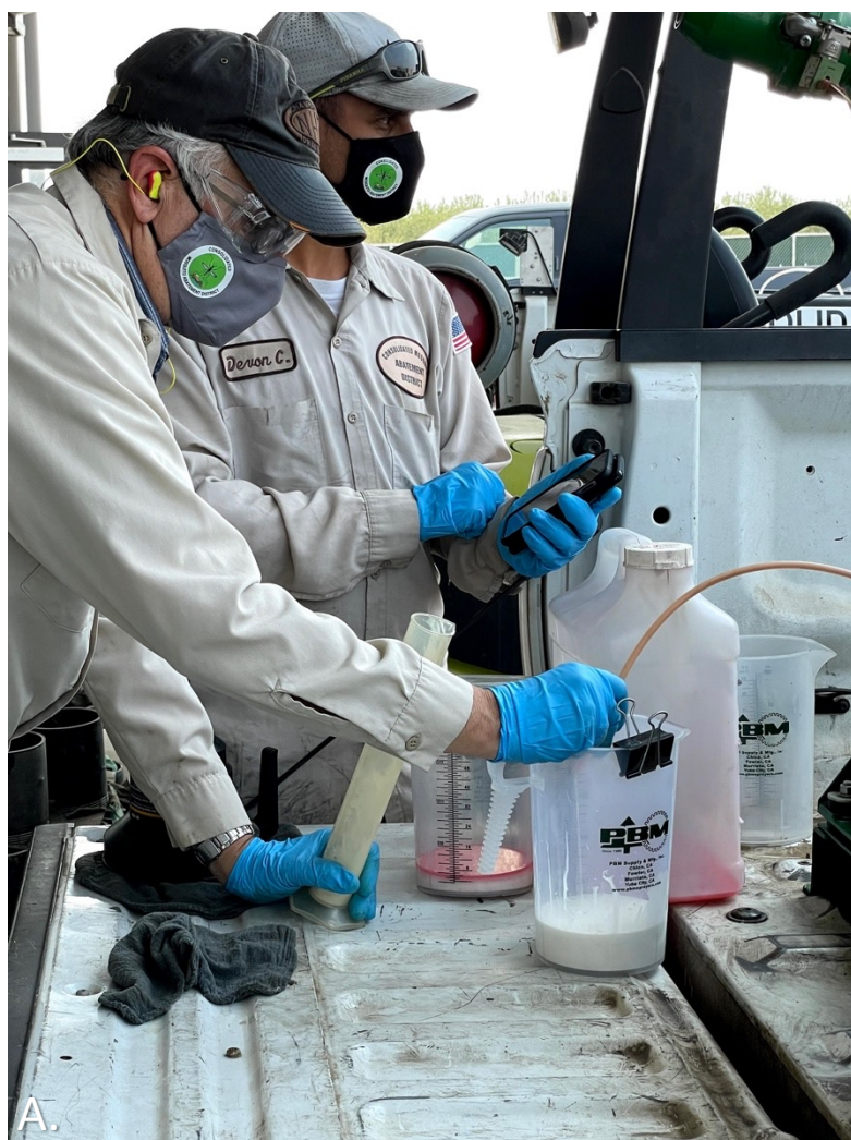
A. Dennis Candito (Adapco) and Devon Cornel (CMAD) checking ULV fogger flow rate. B. Katherine Ramirez (CMAD) setting out caged mosquitoes. C. Steve Mulligan (CMAD) and Denise Candito (Adapco) prepping for equipment calibration.
